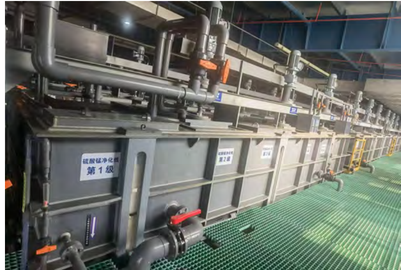
Production Line 2 Deeply purification of Ca from \text{MnSO}_4 stripping solution in Fangyuan Cycling plant (Launched in June, 2022)
