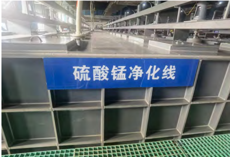
Production Line 2 Deeply purification of Ca from \text{MnSO}_4 stripping solution in Fangyuan Cycling plant (Launched in June, 2022)
