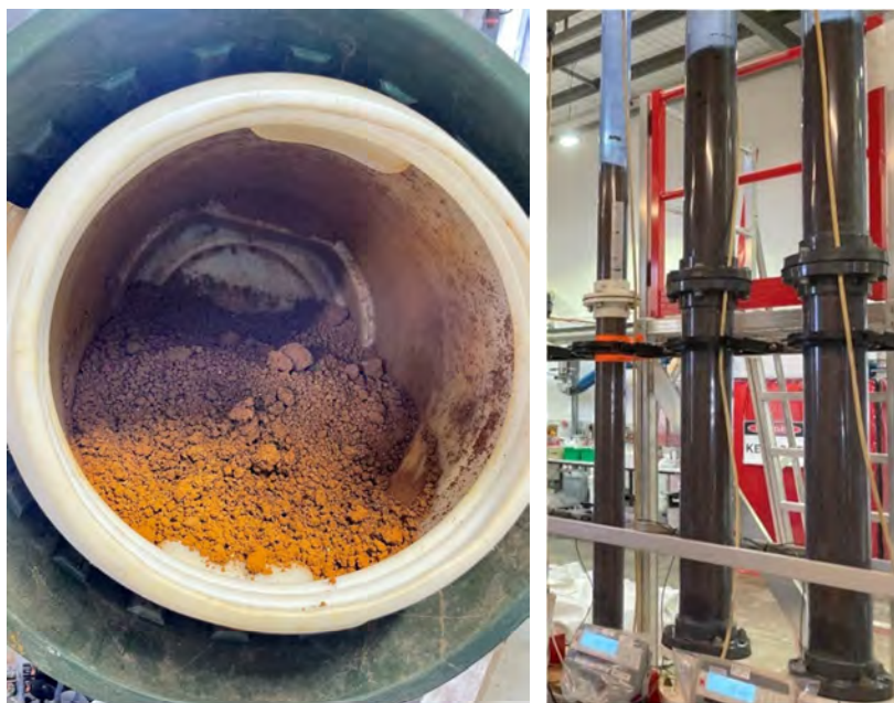
Figure 4: Capital cost of a heap is lower than slurry leach tanks, plus there are benefits to reduction in operating cost through reduction in flocculant and power consumption from dewatering. The material has been successfully agglomerated and percolated on a small scale at ANSTO
