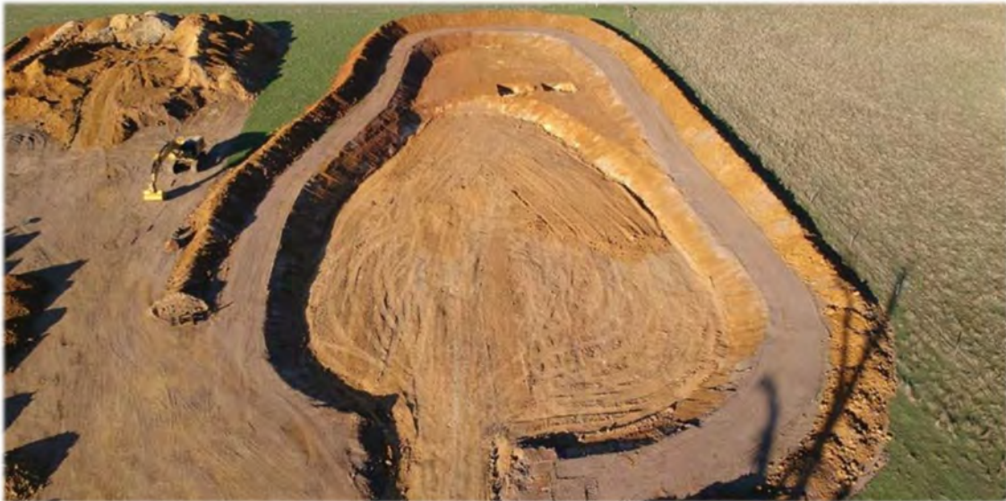
Figure 7: The Koppamurra deposit is within the first 10m, which means that surface mining costs are relatively low compared to other key operating costs such as reagent consumption. This image shows a trial pit excavated at Koppamurra in 2022.
