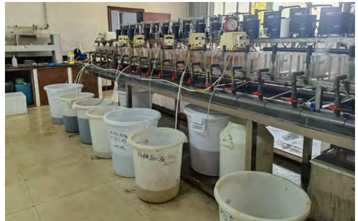
Pilot Scale Line 2 Deeply removal of F from Ni/Co/MnSO 4 solutions by HBL-222 (HT-019-R) (the left one, 15-stage extraction), HBL-221(HT-019-D) (the right one, 10-stage extraction) for Brunp Recycling (conducted during Oct. 2022)
