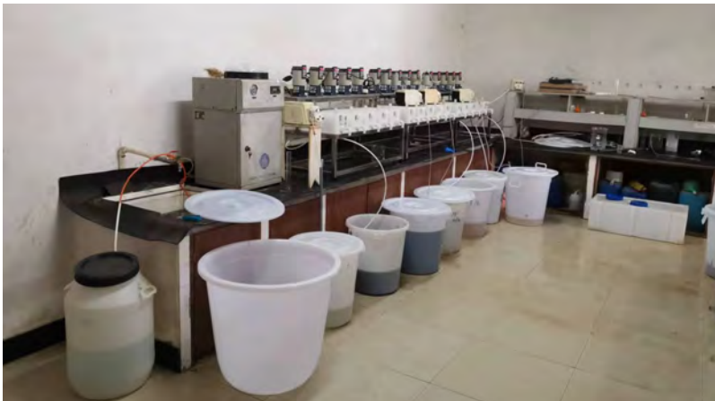
Pilot Scale Line 2 Deeply removal of F from Ni/Co/MnSO 4 solutions by HBL-222 (HT-019-R) (the left one, 15-stage extraction), HBL-221(HT-019-D) (the right one, 10-stage extraction) for Brunp Recycling (conducted during Oct. 2022)
