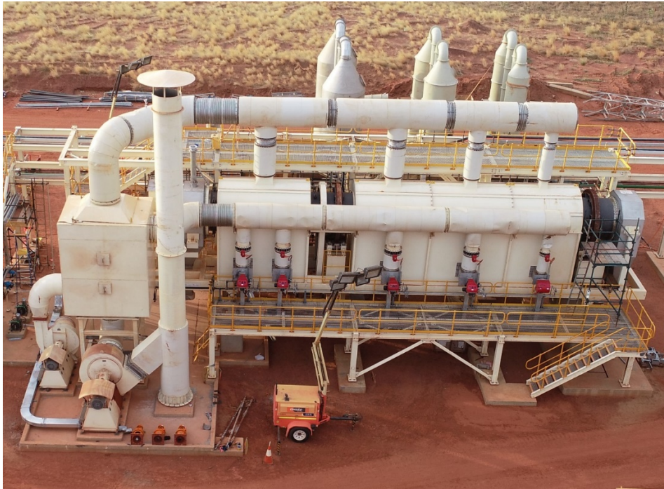
Figure 2 - Indirectly heated rotary kiln
