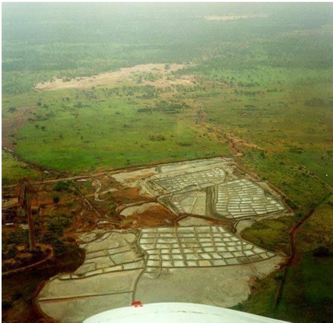
Figure 4: An aerial view of the Kasese pyrite concentrate stockpile before the implementation of the bioleach plant, showing the de-vegetated areas downhill from the stockpile caused by acidic runoff (20)
