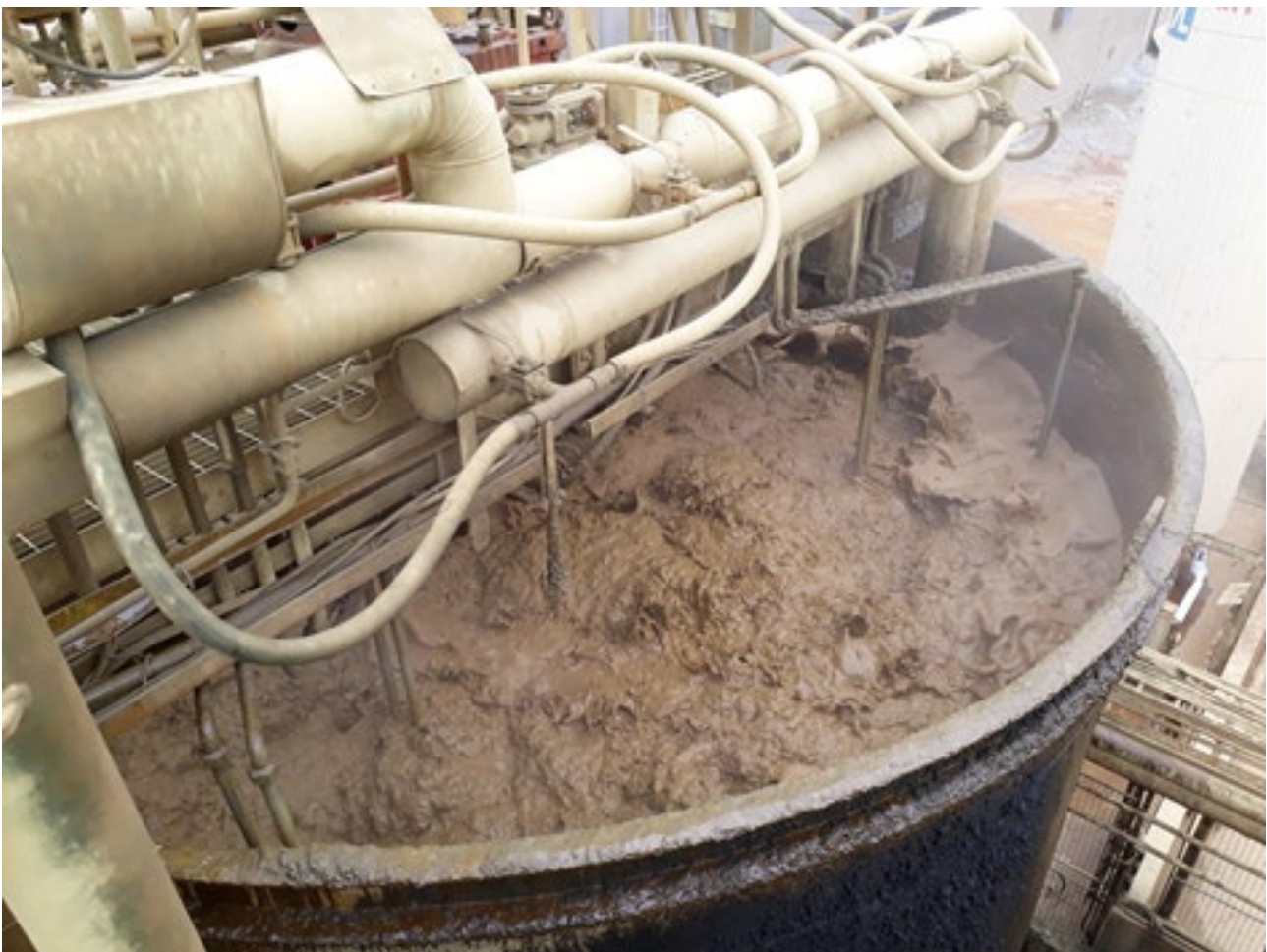
Figure 30: Surface of a primary bioleach reactor at the Mondo Minerals nickel sulphide plant, showing the beneficial impact of antifoam addition to reduce foaming (38)
