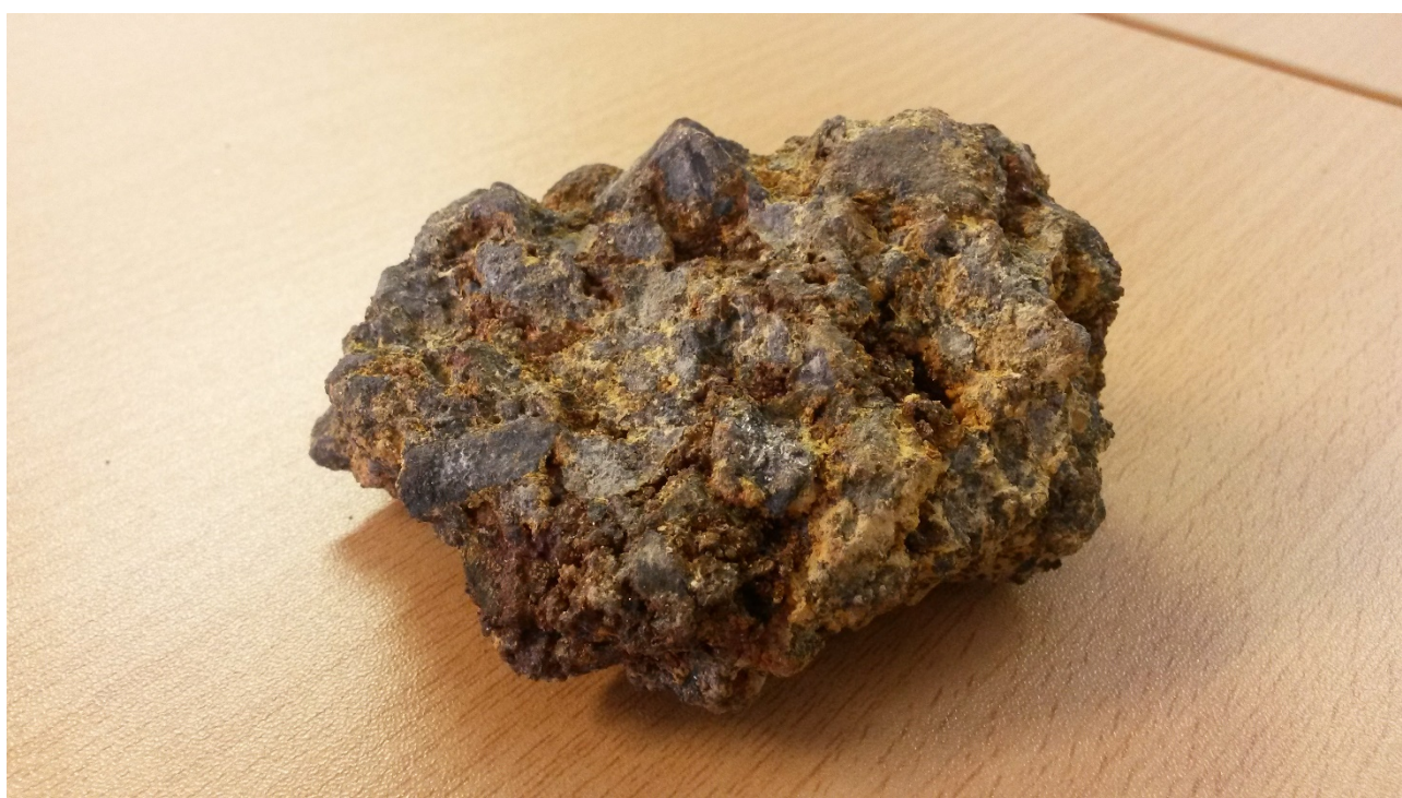
Figure 19: The Terrafame ore after primary leaching, illustrating how it fuses and loses granularity
