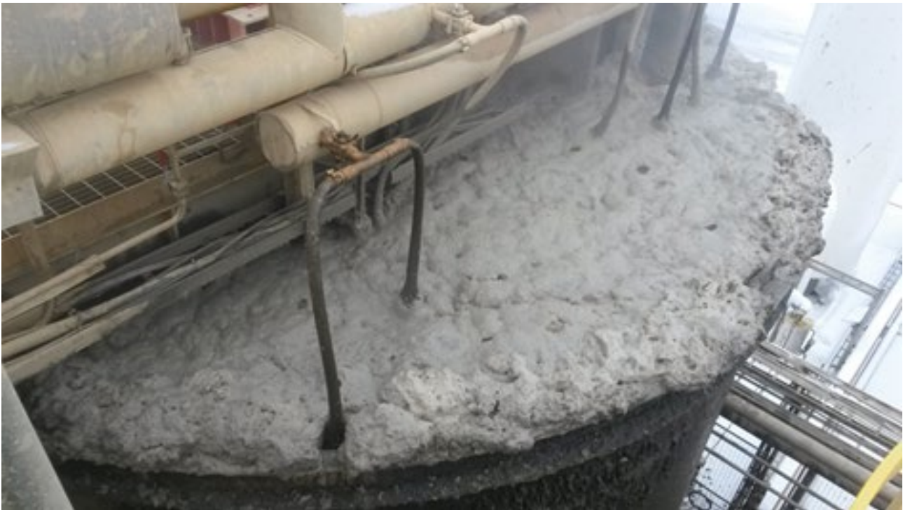
Figure 29: Foaming in a primary bioleach reactor at the Mondo Minerals nickel sulphide plant caused by the presence of talc in the feed concentrate (37)
