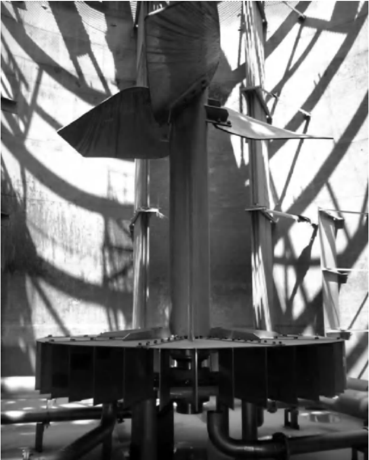
Figure 7: Lower part of the BROGIM ® agitation system utilised in the Kasese bioleach reactors (19)
