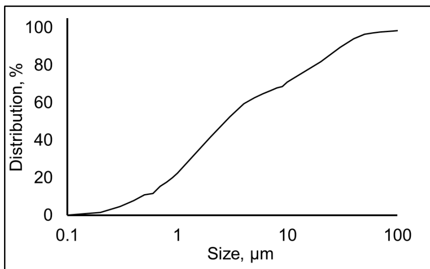
Figure 1 - \text{H}_2\text{TiO}_3 particle size distribution (11)
