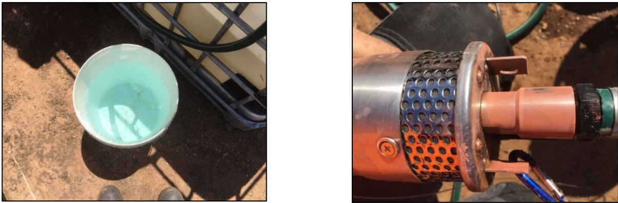
Figure 15 Plates showing groundwater from well KPFR03 and copper coating on submersible pump after tracer test (source – ECR internal technical report)
