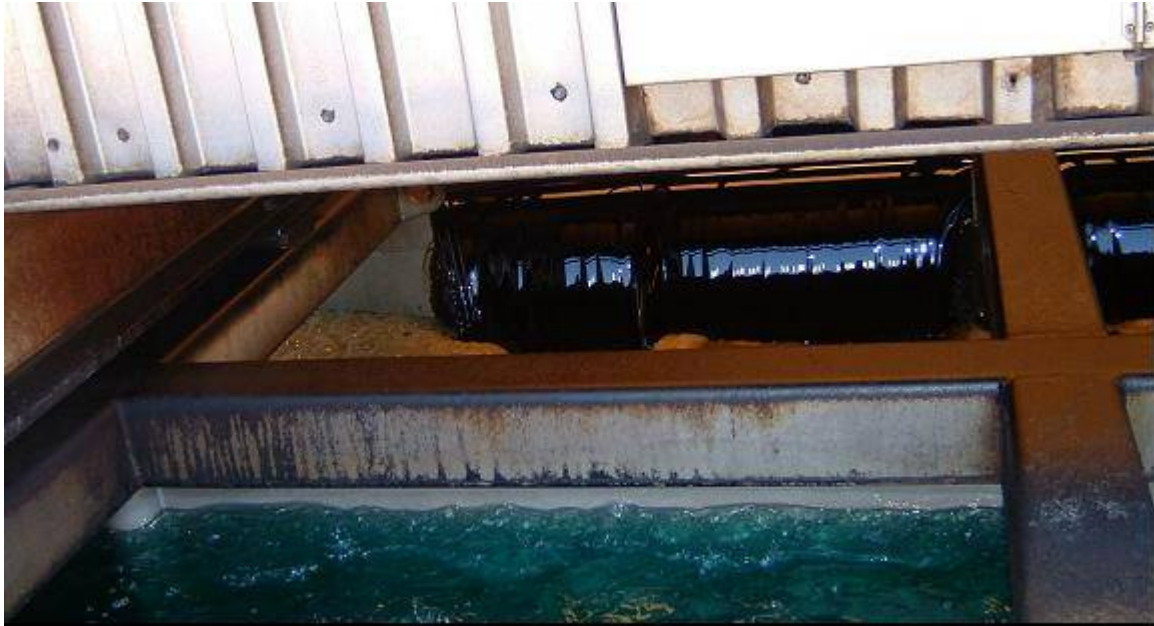
Figure 1. Organic falling +300mm at the weir of a mixer/settler with large amounts of froth generation. The mist created when the bubbles from the entrained air burst is very flammable and can be ignited with a very low energy spark.
