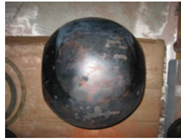
Some coating loss
