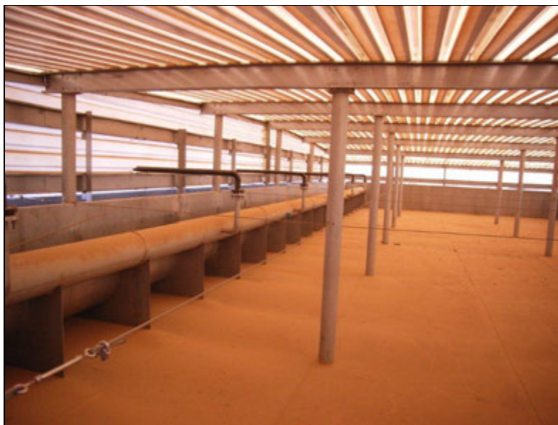
Figure 7: Permanent Crud Removal Piping in a Settler
