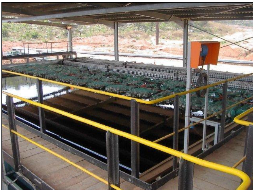
Figure 4: Settler Coalescing Media in use
