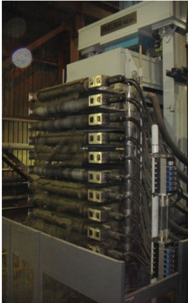
Figure 9: Pneumapress discharging filter cake at HVC.
