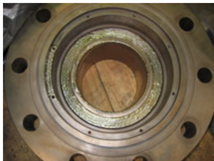
Weld Repaired seat land
