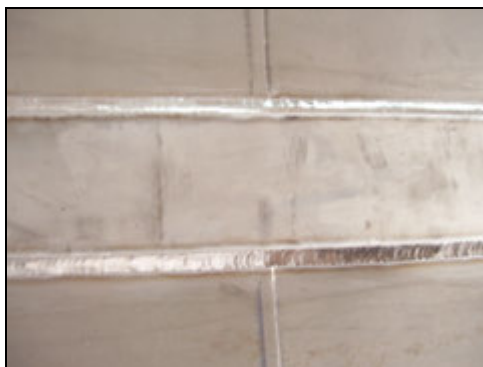
Figure 7: Weld Joints of the titanium strip
