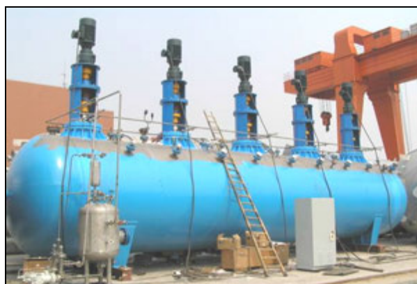
Figure 1: Shop commissioning of autoclave with agitator
