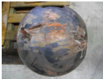
Erosion on ball
