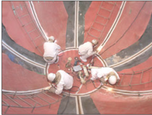
Figure 2: Hemispherical head being welded
