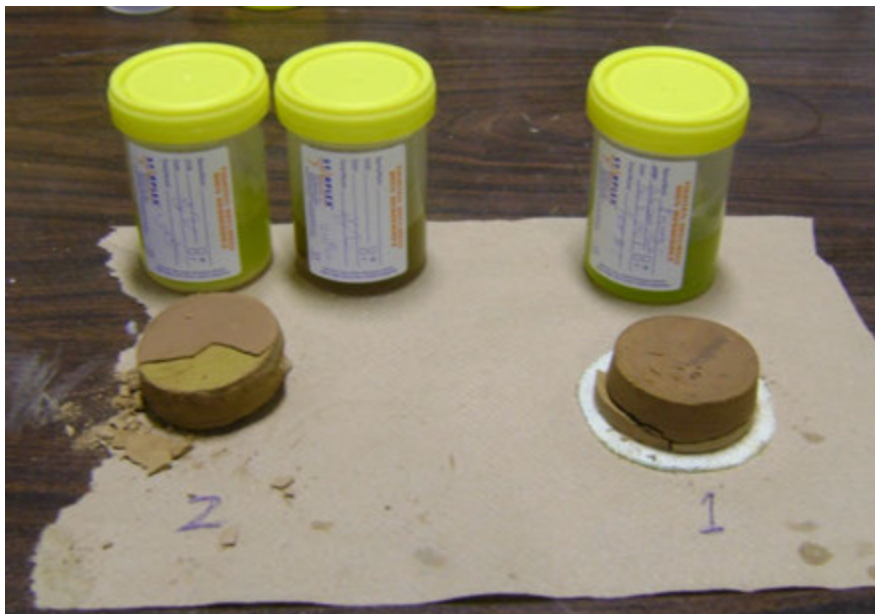
Figure 6: Samples of Autoclave Discharge Cakes, and filtrate and feed slurry.
