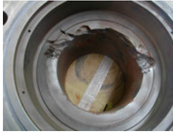
Erosion on Seat Land
