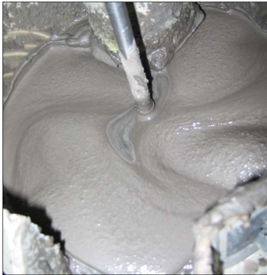
Figure 13: Leach Tank for Coarse Grind Ore P80 = 1.5mm at 68% solids SG (11)
