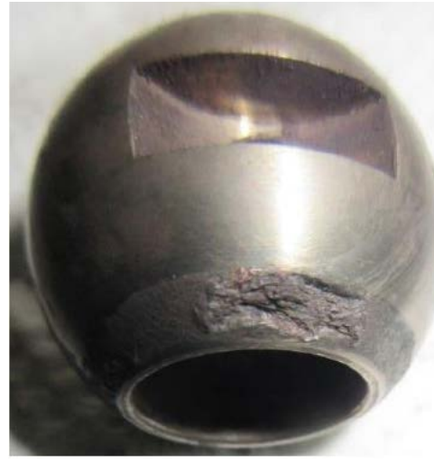
Valve Ball displaying Crevice Corrosion
