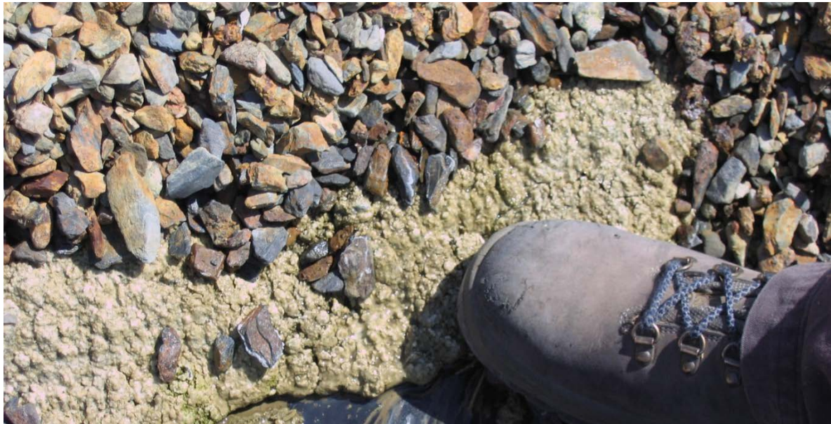
Figure 9: Gypsum precipitate at the toe of an Acid Leach Pad
