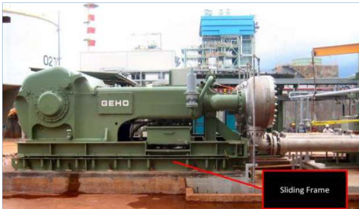
Figure 14 – GEHO® Triplex Pump Sliding Frame Configuration (31) (Photo Courtesy of GEHO)
