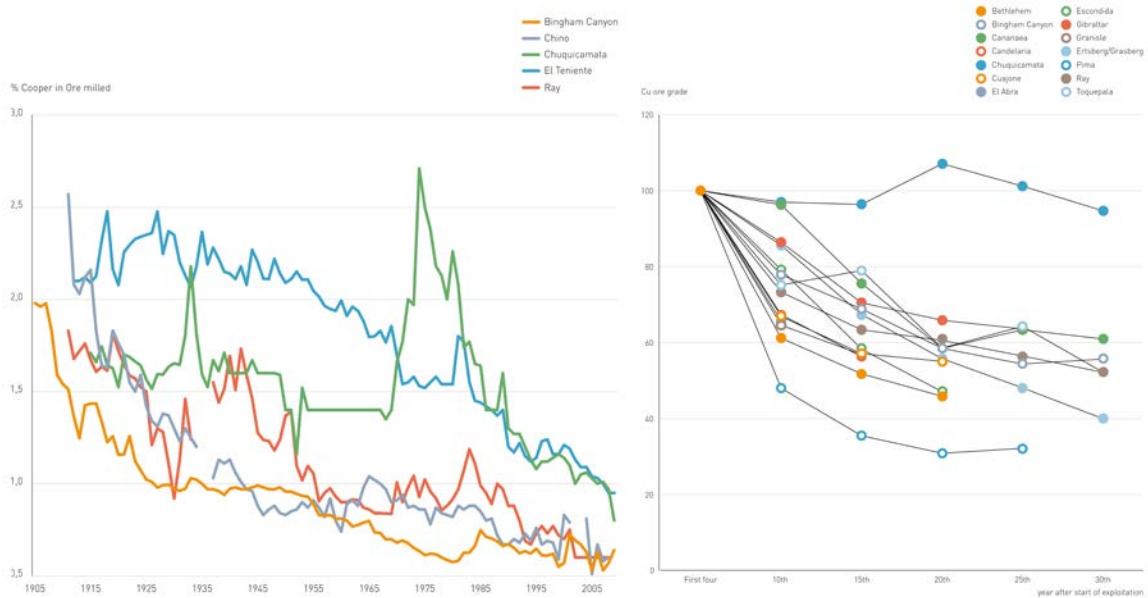
Figure 3 – Long-term Trends in Processed Copper Ore Grades at Specific Mines (15)
